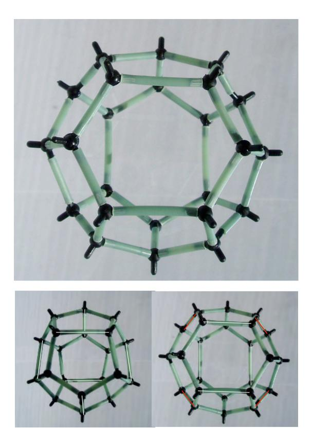
Make measurements on Guy Inchbald's nets. You'll find the edges are of 3 different lengths: the dodecahedron uses 2 of them; the tetrakaidecahedron, all 3. The length of the straw supplied is around 29.5 mm. This (+5.0 mm for the connectors) must be your longest edge (shown white above). Though you can't aim for anything like this accuracy, you'll need to
