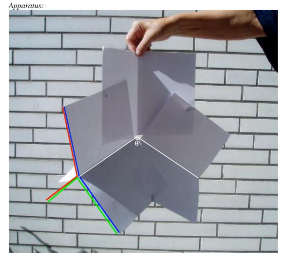
4 120° trigonal prisms made by folding 3 sheets of A4 card width-ways and sticking them together like the red, blue and green sheets shown. 6 paper clips. Each prism represents 3 walls of soap meeting in an edge.
