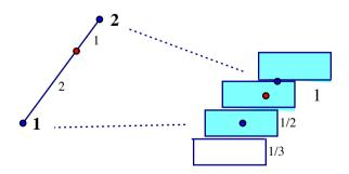
On the left we show that the position of the new centroid divides the line joining the old ones in inverse proportion to the masses. The overhang in the above case  $=\frac{1}{1+2}=\frac{1}{3}$ .
