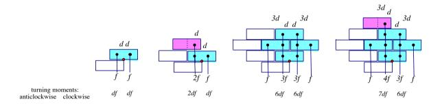
Starting on the left, the blue brick is delicately poised but the addition of the pink brick restores stability. In the third picture, the blue set is again delicately poised and again the addition of the pink brick restores stability. As long as the bricks are absolutely uniform and perfectly positioned, could we continue indefinitely?
