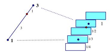
This time the overhang is  $\frac{1}{1+3} = \frac{1}{4}$ . Notice that the new centroid drops half a brick height with every new brick.
