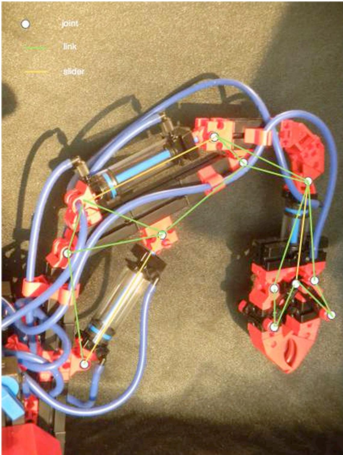
A triangle is a rigid shape so, where three links form a triangle, the piece moves as one and can be considered a single link. On that basis there are 11 joints, 10 links, 3 sliders. Since 1 slider = 1 joint + 1 link, that makes 14 joints, 13 links.  $M = 3l - 2j = 3(13) - 2(14) = 11$ .
