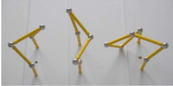
The connection between  $l$  and  $j$  in cases A1, B1, C1 is the same as in the 2-D cases. Complete the table and work out the mobilities [ $M = 3, 6, 9$ ]. The same goes for A2, B2, C2 [ $M = 6, 9, 12$ ].
