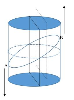
We shear the cylinder parallel to the black plane. The effect is to stretch the circle in the direction AB. The result is an ellipse. The projection perpendicular to the vertical plane through AB looks like this:
