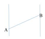
We therefore know that a curve which projects as a circle in plan and a straight line in elevation is an ellipse. We shall need this fact shortly.
