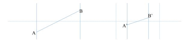
The figure has been uniformly compressed vertically so that the projection is still a straight line.
